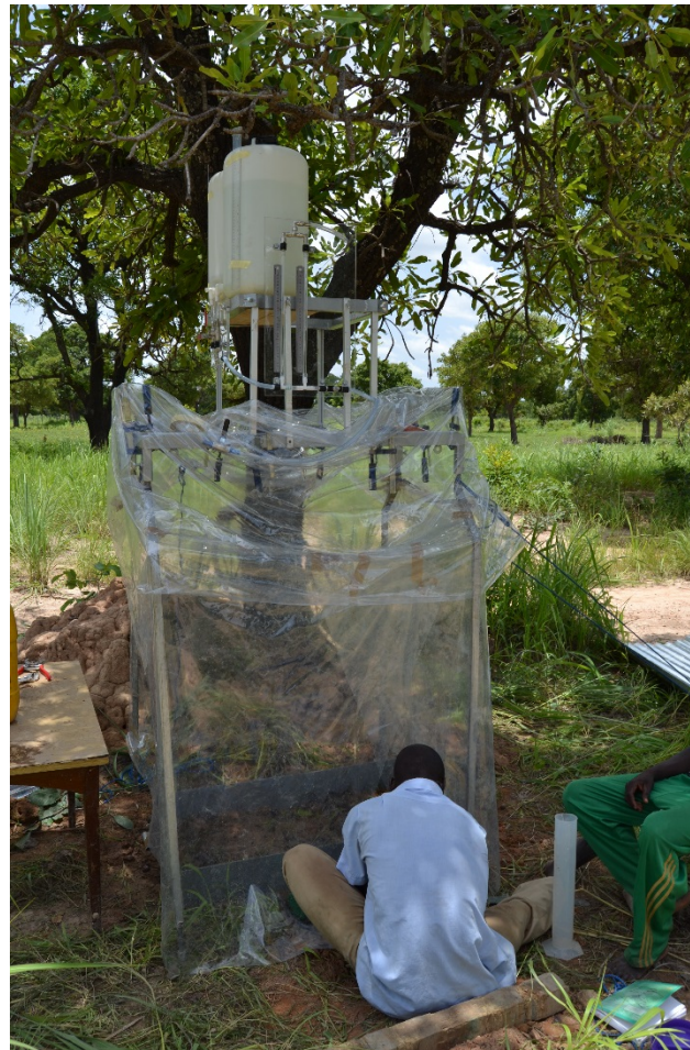
Soil infiltrability measurements: Drip-type Amsterdam rainfall simulator
